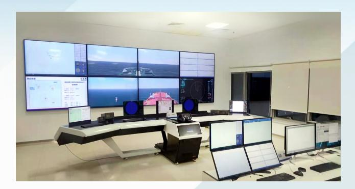
CCS has established intelligent ship simulation test and verification platform, which is capable of high precision hardware-in-the-loop simulation test. The platform, being equipped with a test scenario database on the basis of rules, accident recurrence and real traffic flow, provides qualitative and quantitative assessment of intelligence capability, behavior safety level and economy. The platform also allows for expert and Al accompany modes to make such tests more rational and science-based.
