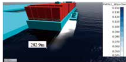
Figure 5: The spread range of the combustible gas when LNG leak to the refueling station (the north wind, volume concentration 2.5% ~ 15%)
