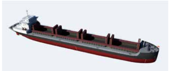
Picture 9 The concept sea-river ship for specific route: 20000 ton bulk carrier
