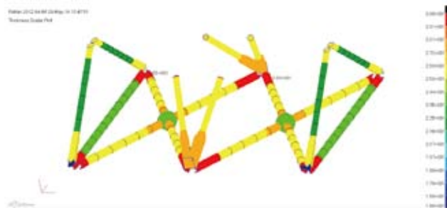
Figure 2: diagram of as-built thickness of lateral brace and diagonal bracing of the unit
