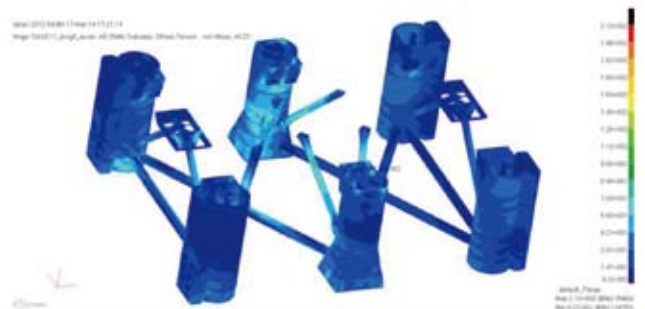
Figure 5: maximum stress of unit's strut system (storm self-existence, load characteristics is the longitudinal acceleration)
