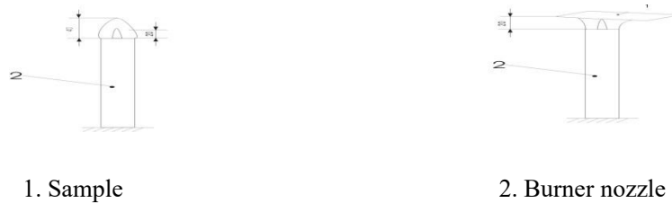
Fig.1 Schematic diagram for devices used for flame retardation test on dressing belt and belt buckle materials
