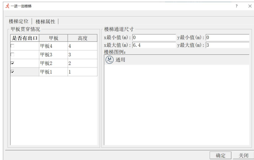
Figure 6.3.2.2(2) Set the location of staircase
