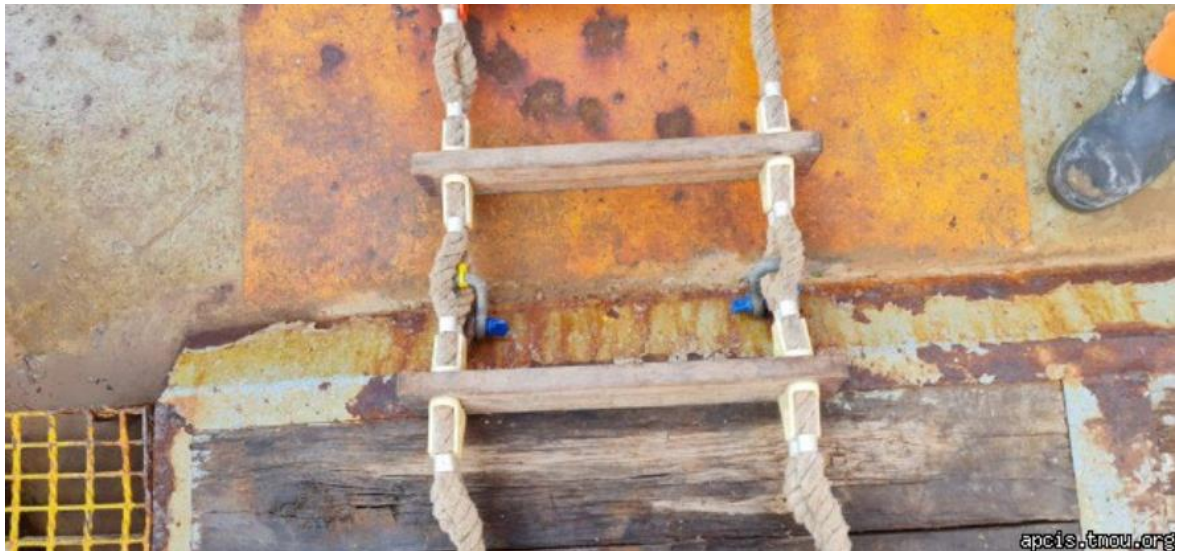
Picture 7 Unsafe pilot ladder securing arrangements
