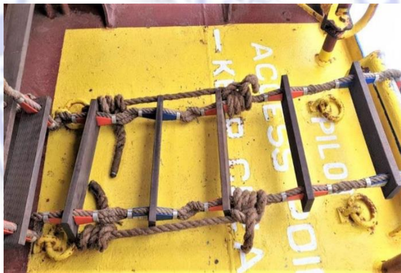
Picture 2 appropriate application of rolling hitch knot to secure a pilot ladder to a deck strong point (Source: AMSA Marine Notice 2023/04)
