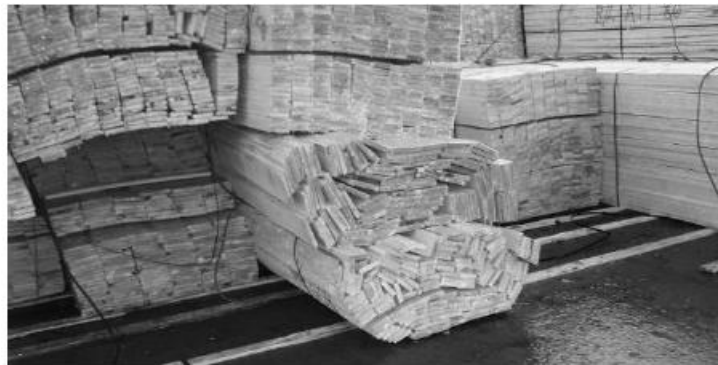
Figure 6.2. Example of poor rigidity
