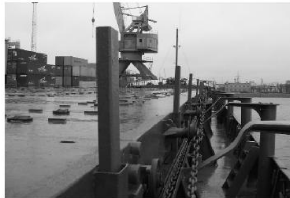
Figure 6.7 Example of uprights for bottom blocking
