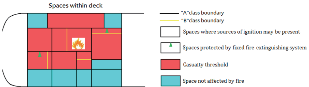
Figure 1.5.2(2)b Not protected by fixed fire-extinguishing system
