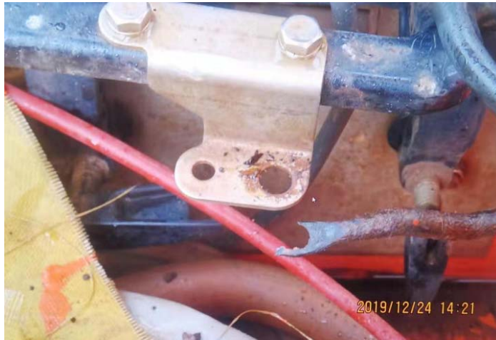
Rescue boat rudder turning handle corroded and broken
