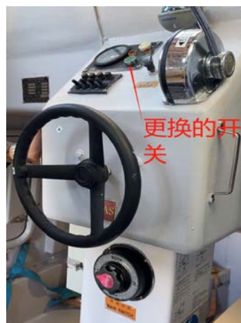
Life boat engine defective ( Starting button renewed)
