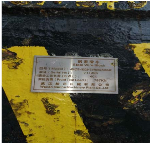
Cargo handling equipment does not marked S.W.L.(rectified)
