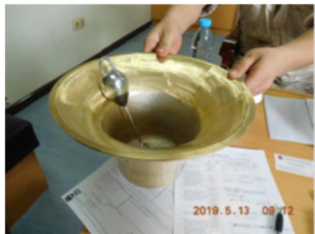
Bell diameter less than 300mm and not meet requirement
