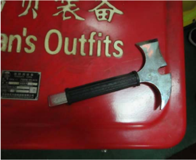
Handle of fire-fighting axe not insulation
