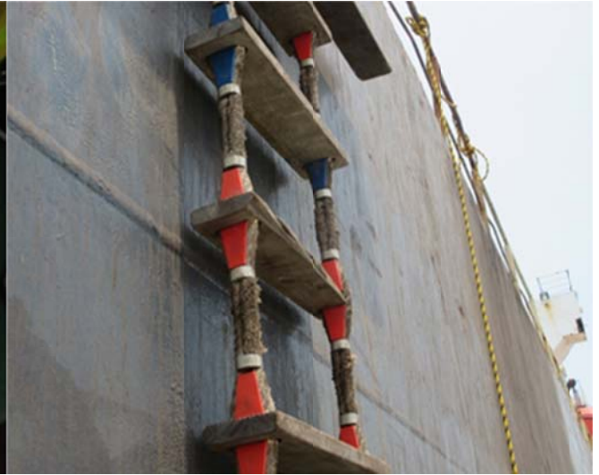
Step of pilot ladder damaged
