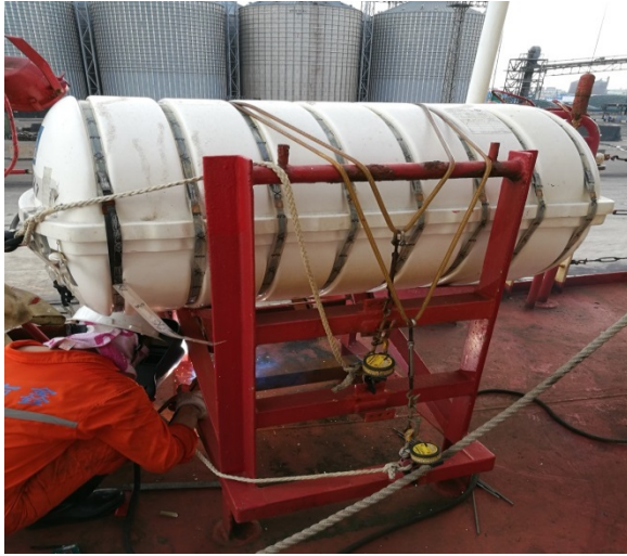
Life rafts were fixed improperly
