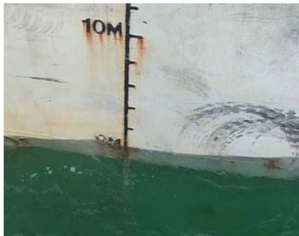
Unclear load line mark
