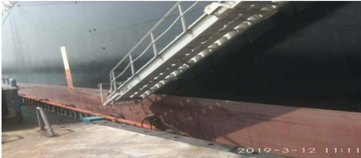
Gangway is not provided with safety net
