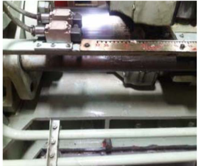
Steering Gear Hydraulic Heavy Leaking
