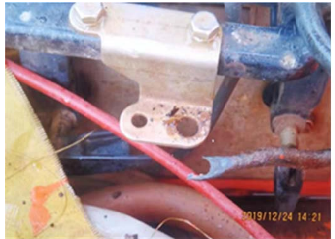
Rescue boat rudder control lever damaged
