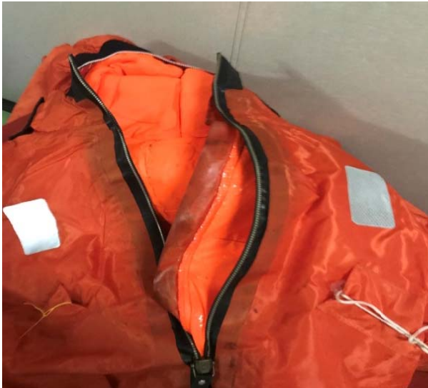
Immersion suits are severely deteriorated
