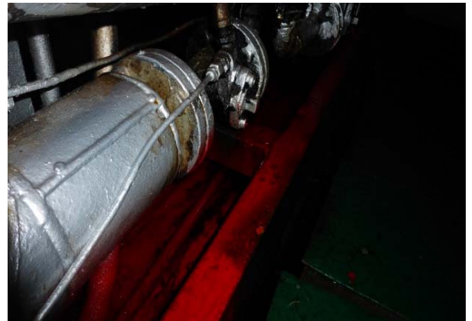
Main engine fuel supply unit oily seriously
