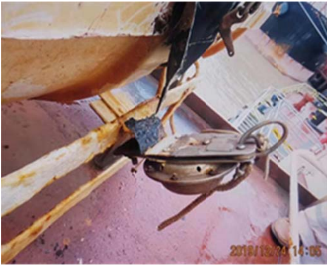
Foundation of liferaft HRU fractured
