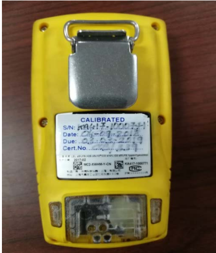
Gas detector calibration overdue.
