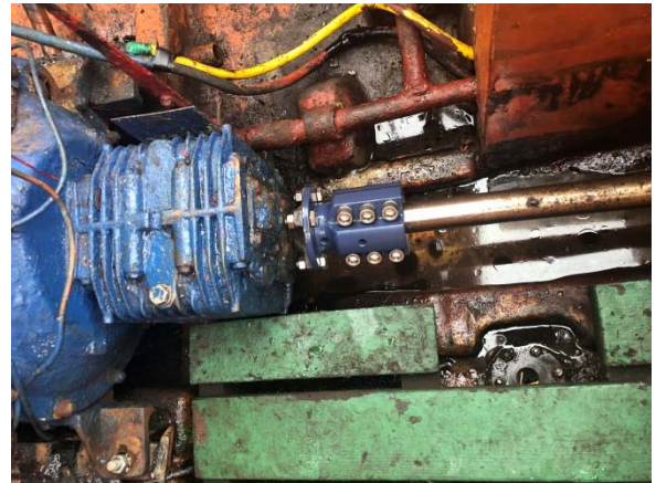
Propeller shaft of rescue boat broken(repaired)
