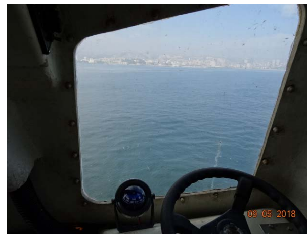
The window of the free fall lifeboat not clear (already replaced)
