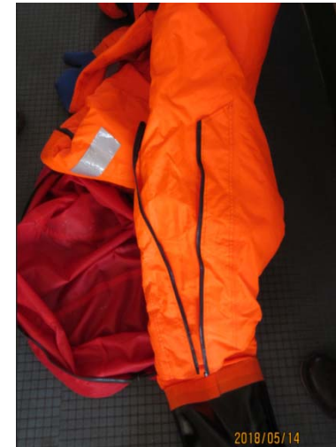
Damaged zip on immersion suit
