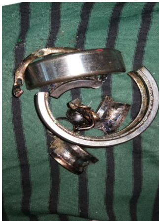
Bearings of emergency fire pump damaged
