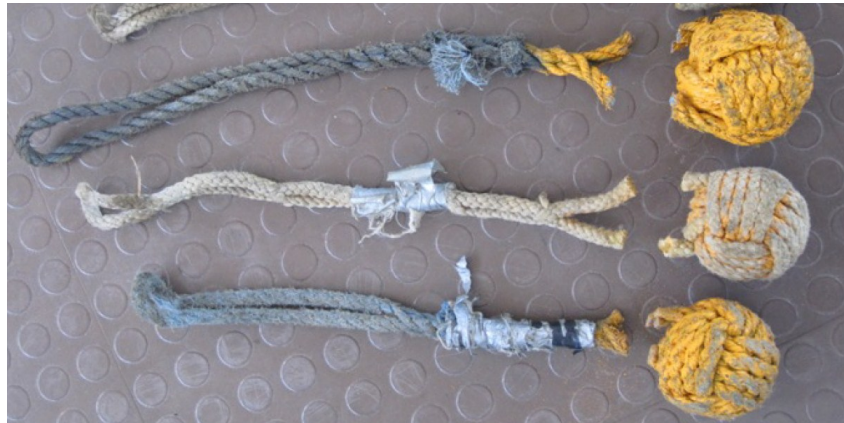
Unacceptable monkey's fists containing inappropriate weighting material removed from service
