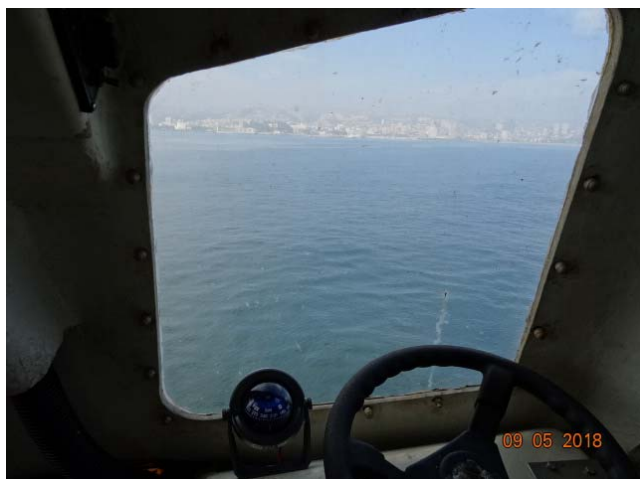
Window glass on life boat dirty (renewed)
