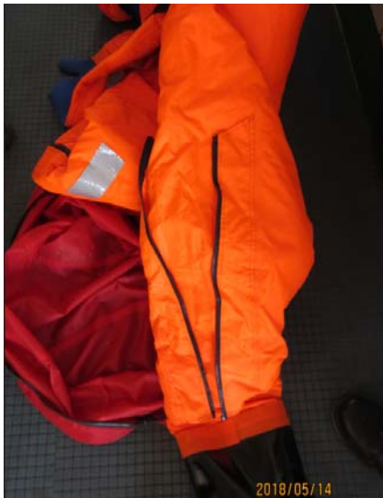
Slide fastener on life jacket damaged.
