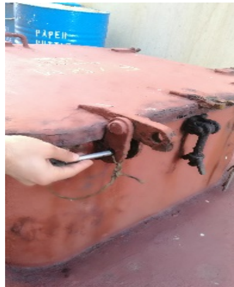
Securing pins for hatches on main deck (ER and Hold) missing.
