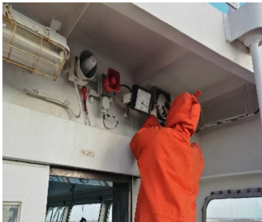
The RPM indicator (bridge and bridge wings) shows not actual situation.
