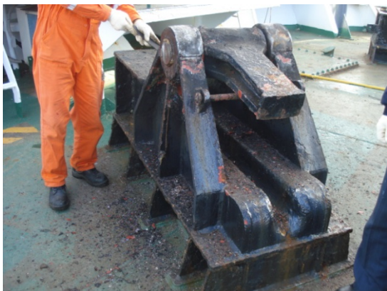
Chain stopper is seriously corroded.
