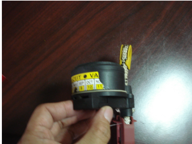
Hydrostatic release unit for life raft has expired.
