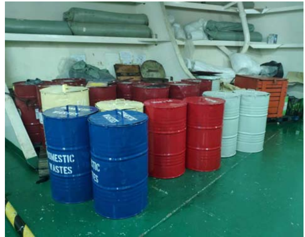
Several items stored in steering gear room not secured properly
