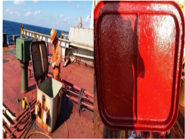
Booby hatch cover sealing gasket defective
