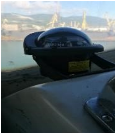
Compass in life boat leaks liquid (after renewal)
