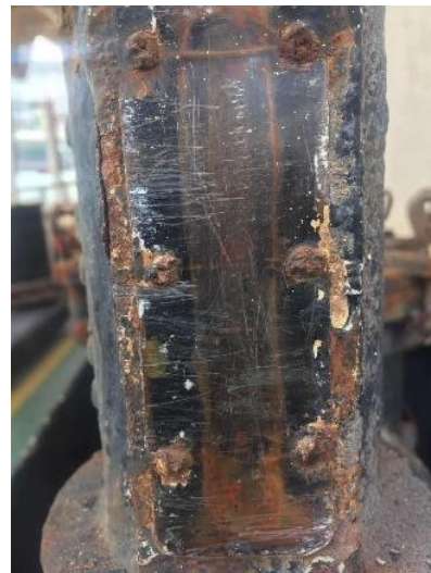
bunker line on deck and ER indicator of position unreadable
