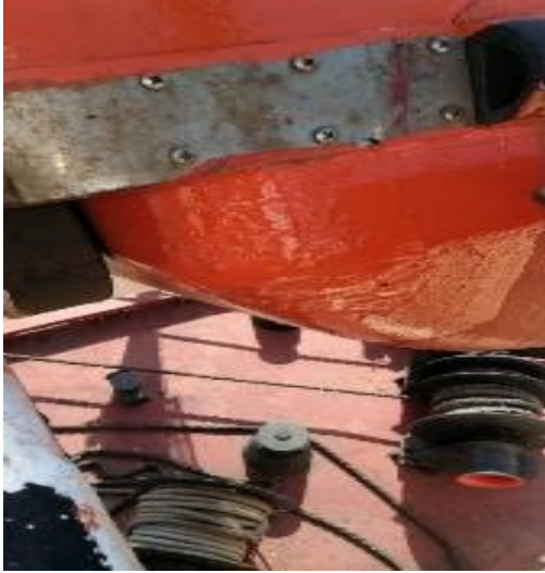
Free fall lifeboat stern corner-damaged (repaired)
