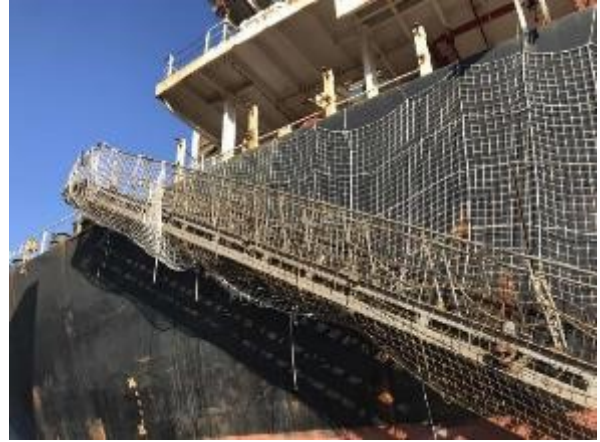
Accommodation ladder no safety nets (rectified)
