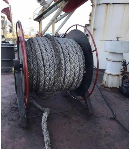
Drums for mooring ropes corroded, handles damaged
