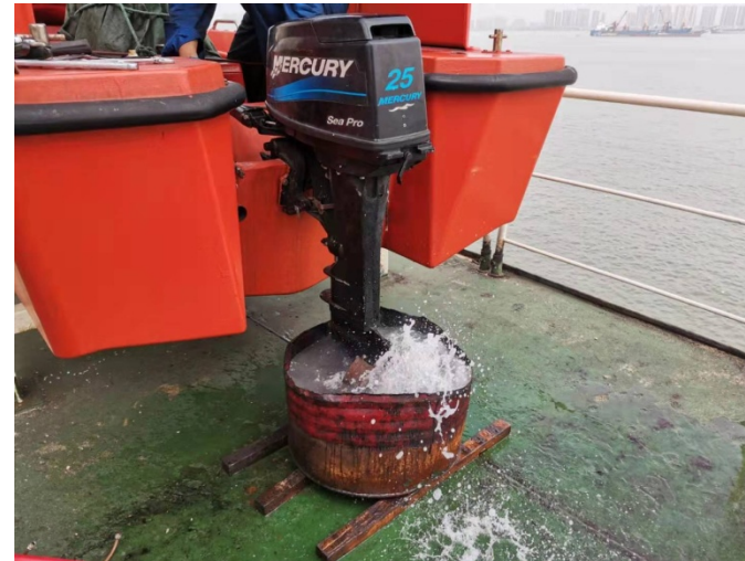
Rescue boat engine starting failure (rectified)
