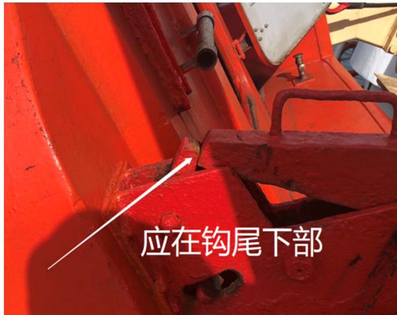
Freefall lifeboat release system defective
