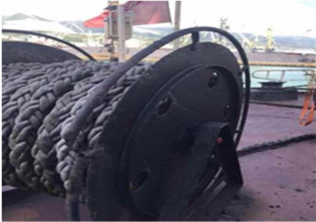
Drums for mooring ropes corroded, handle damaged
