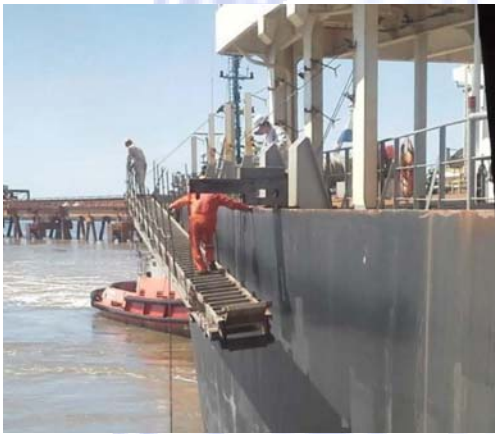
Crew on the accommodation ladder while hoisted. Accommodation ladders safety nets not fitted
