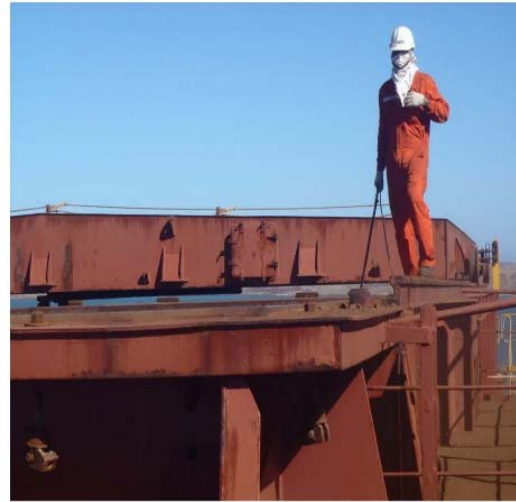
Working on open hatch cover without fall protection
