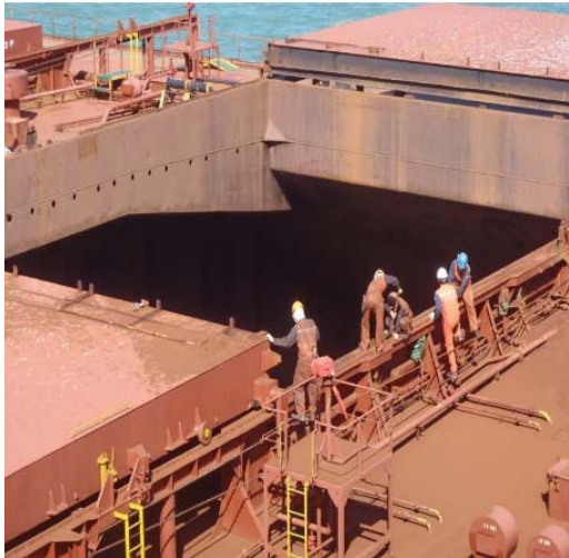
Working on open hatch cover without fall protection
