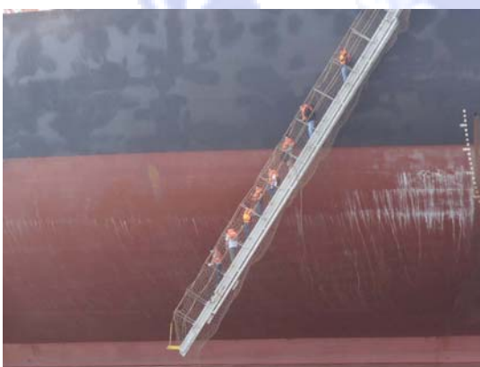
Accommodation ladder incline > 55^\circ
