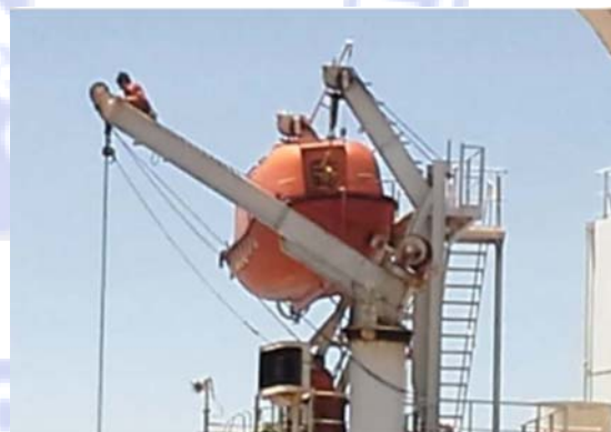
Working at height without fall protection
