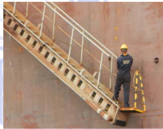
Crew on the accommodation ladder while hoisted. Accommodation ladders safety nets not fitted
