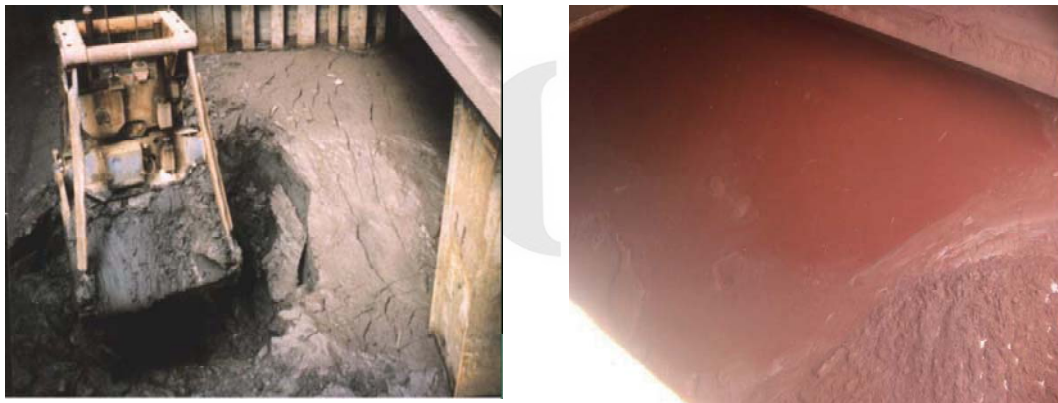
Figure 1 Cargoes liquefied and moisture migration
