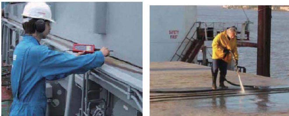
Figure 5 Tightness test to hatch covers (ultrasonic test and hose test)
