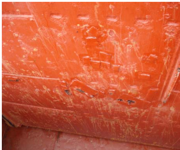
4-1 Holed hatch covers, attention to be paid to the lower part of the cover panels and the ventilators or cement holes in panel(if any)
