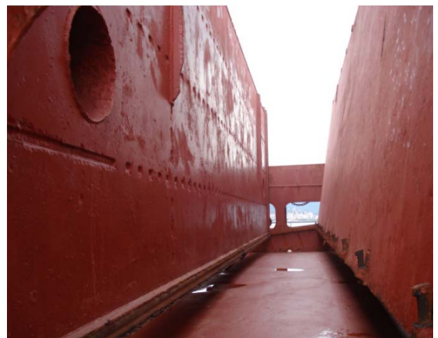
4-1 Holed hatch covers, attention to be paid to the lower part of the cover panels and the ventilators or cement holes in panel(if any)
