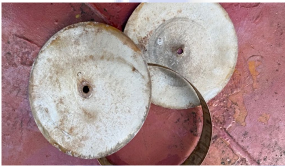
Severely damaged float disc
