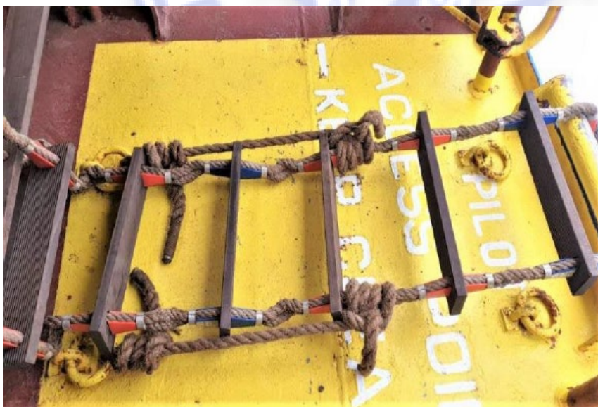
Figure 7 Pilot ladder secured to approved main deck strong points using rolling hitch knots.
