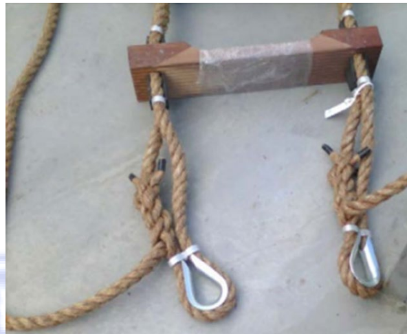
Figure 4 Side ropes with splices (connections)
