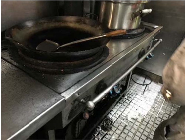
The pan using fuel oil in kitchen is in fire danger and shall stop using it
