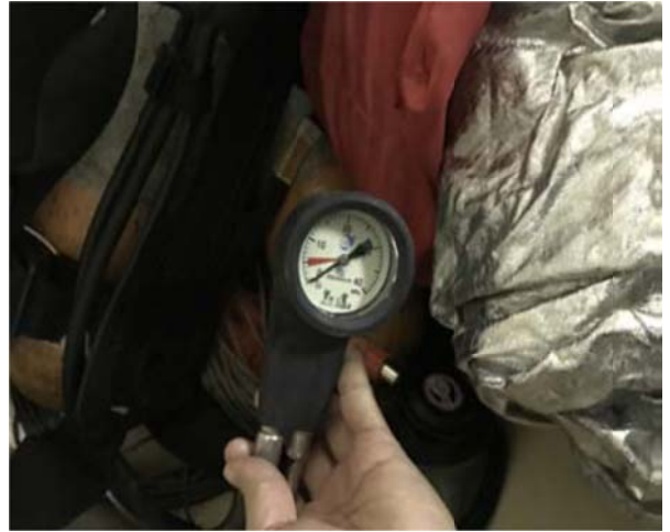
Failure occurs to the low pressure alarm of fireman's outfit SCBA
