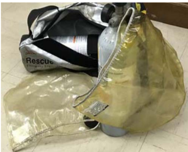
Aging failure occurs to the EEBD mask in steering room
