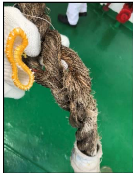
The rope of port lifeboat is seriously corroded
