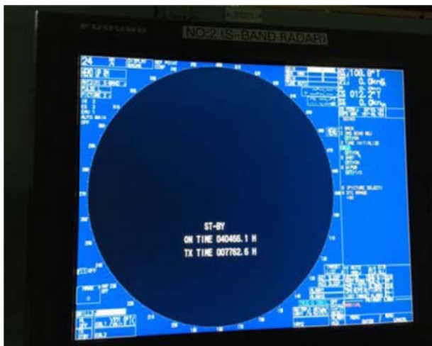
The actual service time of radar magnetron exceeds the time specified in the Product Specification
