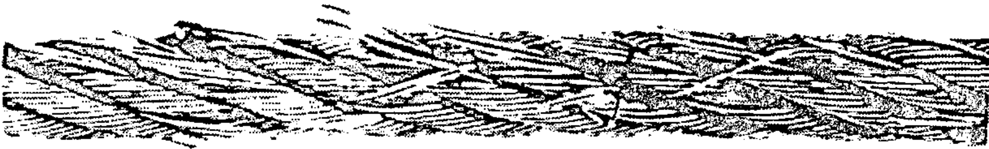
FIG. 9. EXAMPLE OF DISTRIBUTED CROWN WIRE BREAKS.
