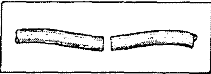
FATIGUE FAILURE-STRAIGHT ACROSS
