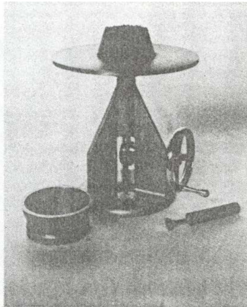
Figure 1.1.2 – Flow table and accessory apparatus
